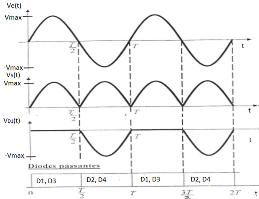
Figure 6 redressement double alternance
