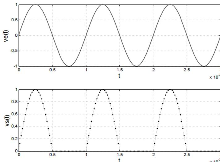
Figure 2 redressement simple alternance
