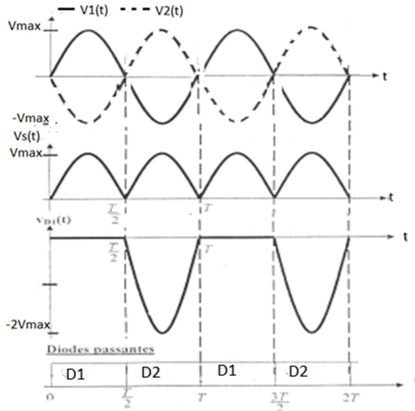
Figure 4 redressement double alternance
